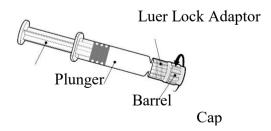
Hold the syringe by the barrel, not by the plunger. Unscrew the syringe cap by twisting it anticlockwise.
